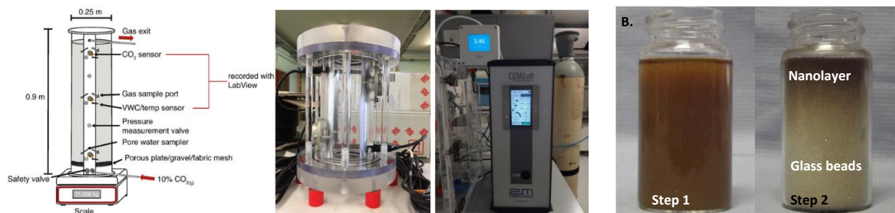
Figure 1. Left: decimetric column and schematic diagram (left), and column before assembly with the CEMLab gas generator / mixer (Center, MIMAROC platform, BRGM); and right: porous medium with controlled distribution.
